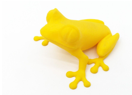
Pict. 29 - the 50-microns treefrog is commonly used as a 3D printing benchmark.
