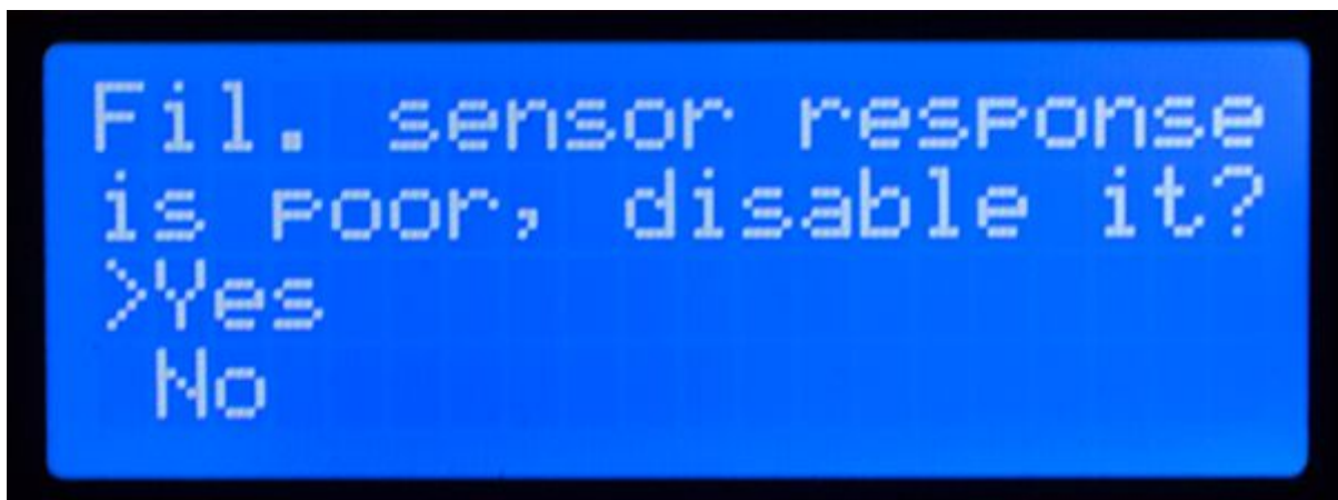
Pict. 38 - Information about filament quality (Filament sensor engine 2.0)
